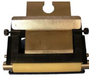
H-100 guide (inverted) with plane iron
